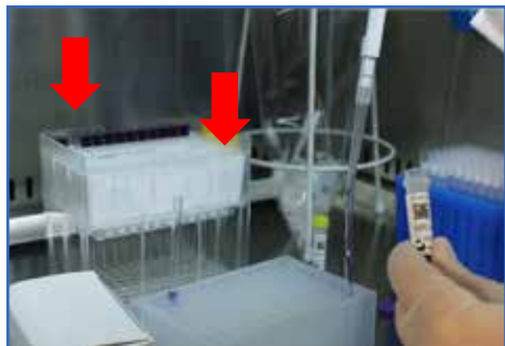
Prepare 2 NMR tubes with quality control solution and place controls at positions A2 and H12.
